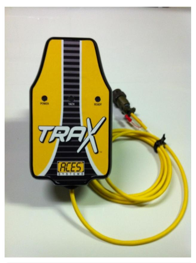
The ACES Systems' Model 550 Optical ACES TraX is a state of the art, semi-permanently mounted optical camera that automates the task of obtaining accurate blade track data when used in conjunction with certain ACES Systems' analyzers.
